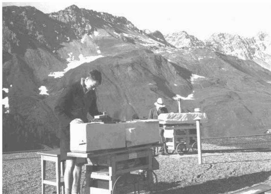
Fig. 6 Total ozone measurements at Arosa, Switzerland, during an intercomparison around 1952. Historical total ozone data such as the series from Arosa, which goes as far back as 1926, provide important information on the past variability of the stratosphere (Source: LKO Arosa, MeteoSwiss).
