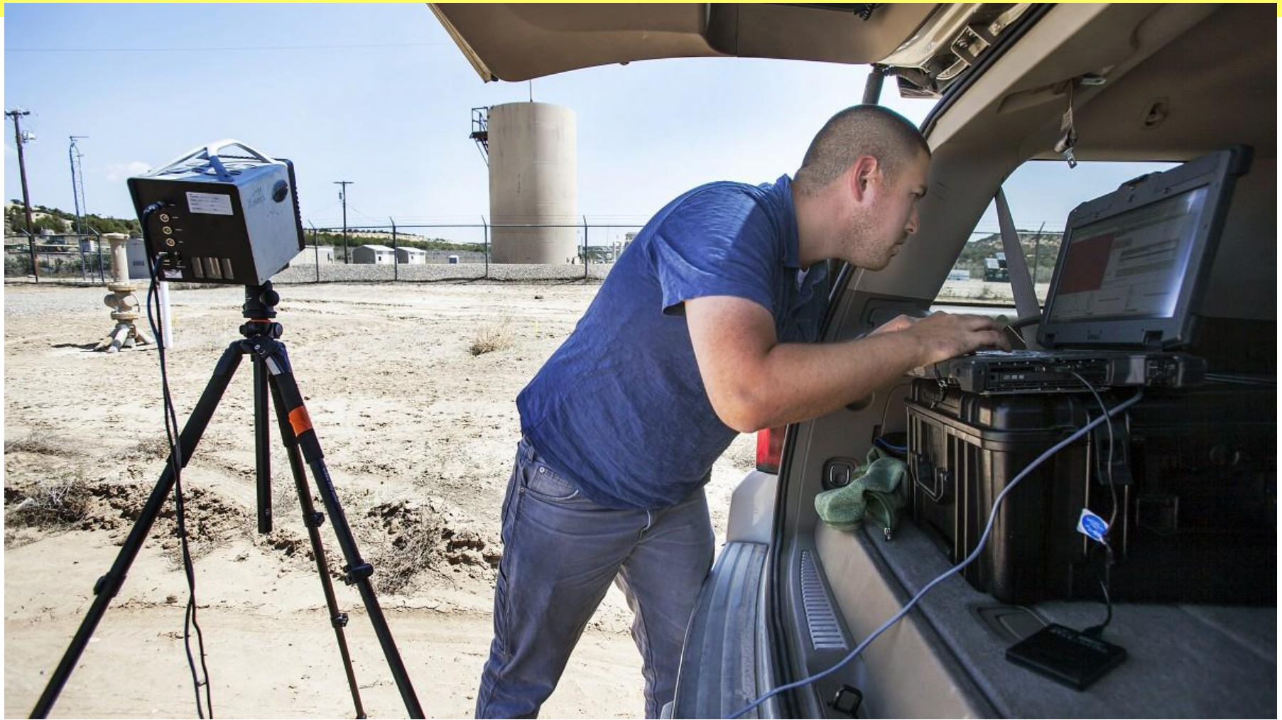
NASA CAMERA — Andrew Thorpe of NASA's Jet Propulsion Laboratory powers up a thermal camera imaging system next to a storage tank believed to be leaking methane at a natural gas facility near Aztec, New Mexico. Photo by Shaun Stanley
