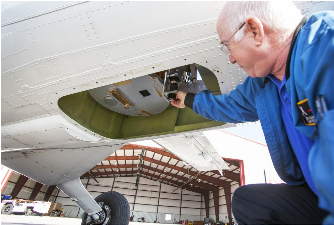
Seth Chazanoff of NASA's Jet Propulsion Laboratory conducts final checks on a Hyperspectral Thermal Emission Spectrometer mounted within an aircraft used to study methane gas emissions in the Four Corners area. Photo by Shaun Stanley
