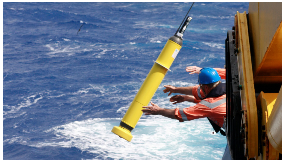
Fig. 12. An Argo float being deployed to measure ocean temperature to depths of 2,000 meters.
