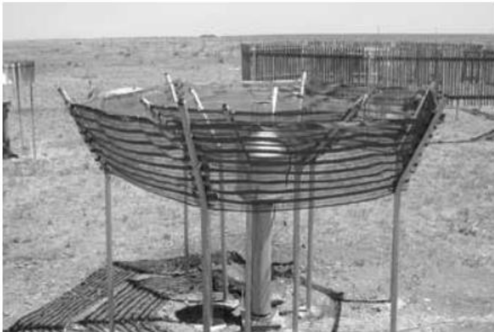
Figure 4—The catch efficiency for the half-scale Wyoming windshield drops rapidly as wind increases.
