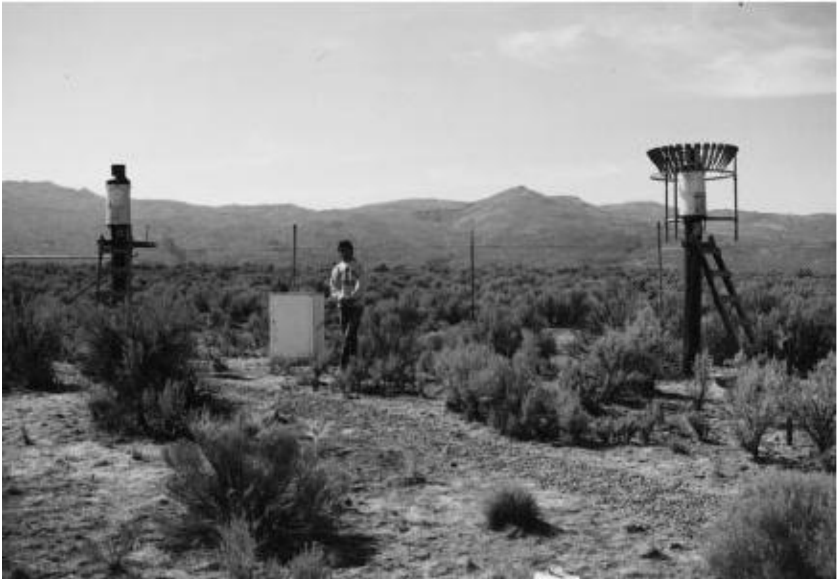
Dual-gauge measuring system (bridled shield and unshielded universal recording gauges) Idaho.
