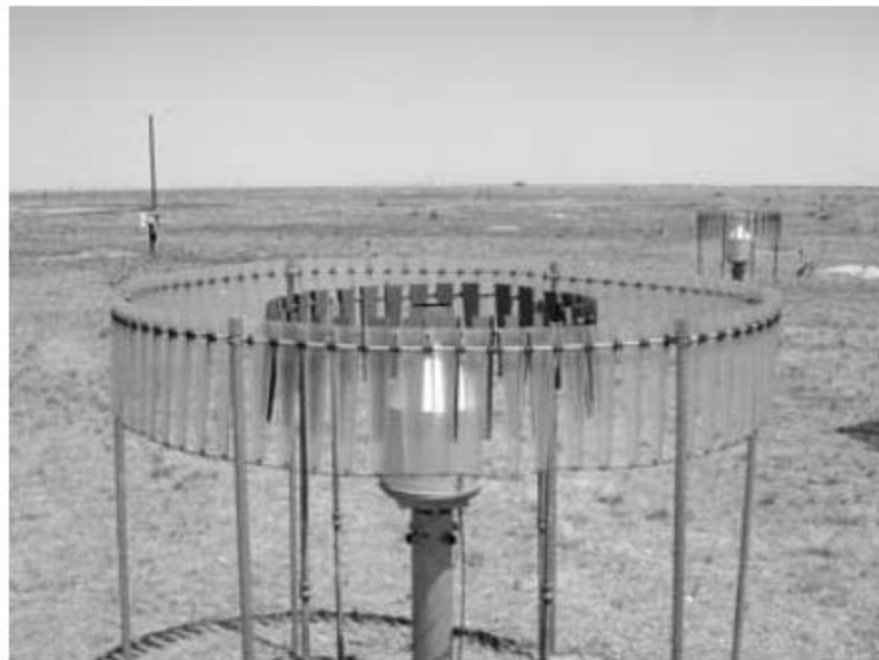
Figure 3—The double Alter windshield performs well in high winds.
