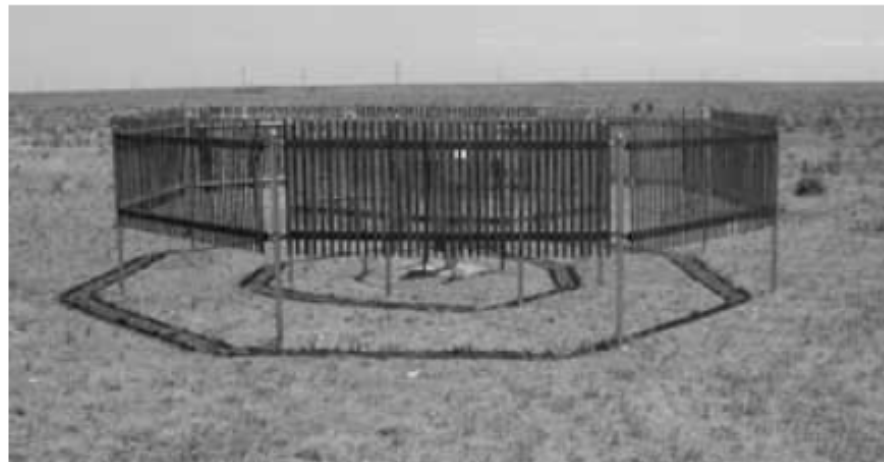
Figure 1—The double fence intercomparison reference gauge catches 92 to 96 percent of the precipitation that falls.
