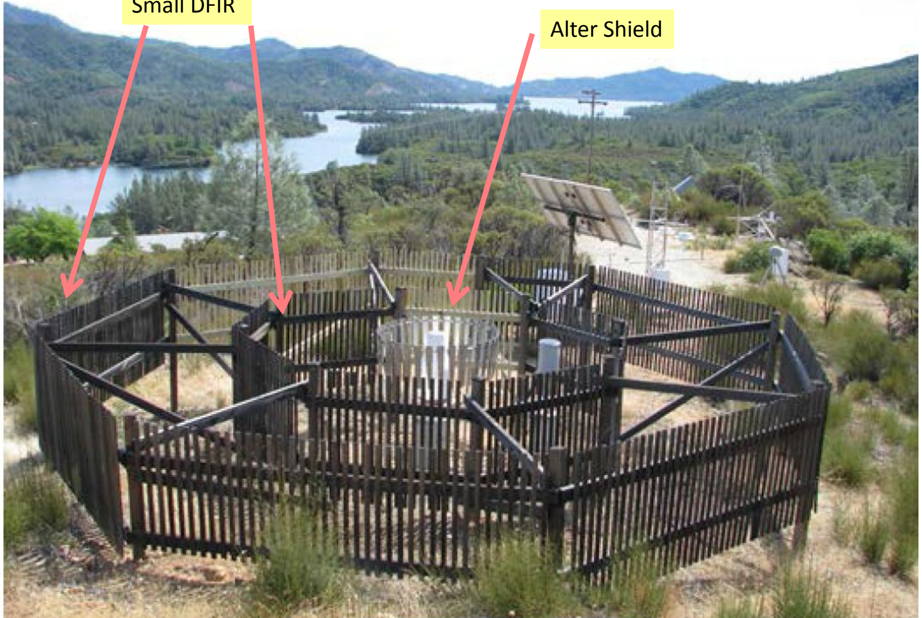
USCRN Geonor-T200B gauge within both a Small double fence Intercomparison Reference <Small DFIR> shield and Alter shield, near Merced, CA...
