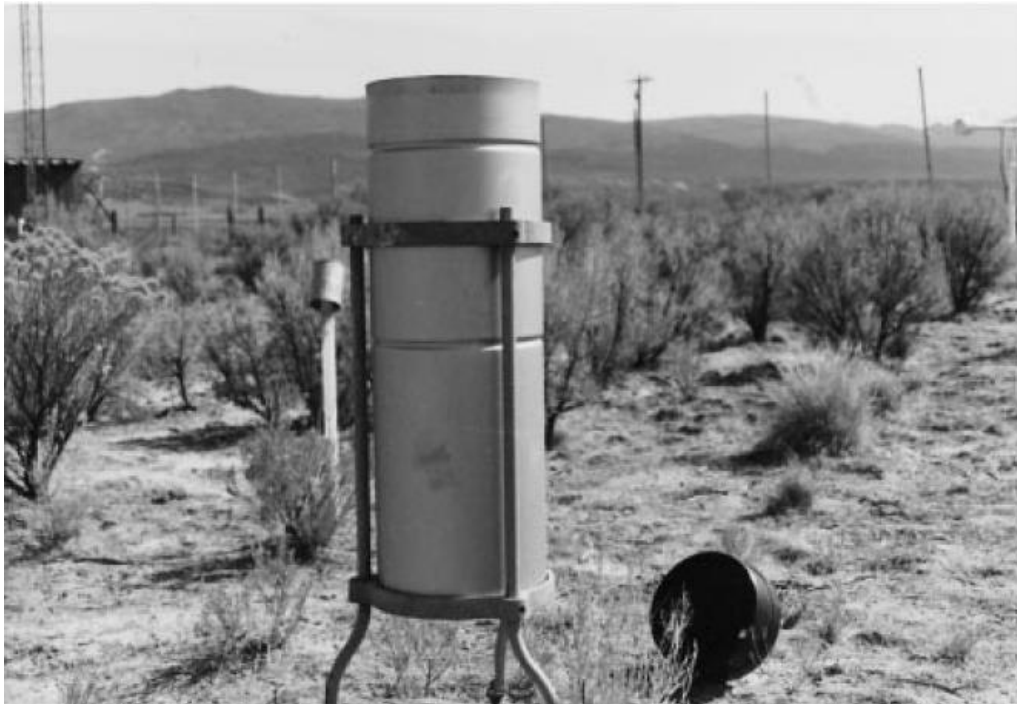
8-inch unshielded gage in Idaho where some of the intercomparisons were done.
