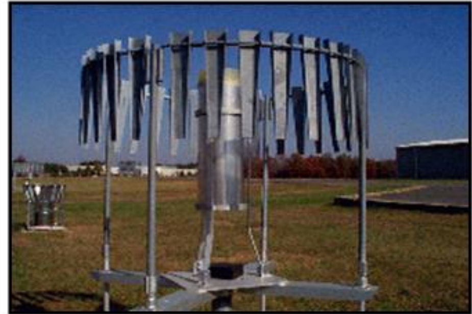
Figure 5 NWS 8-inch Manual Gauge
