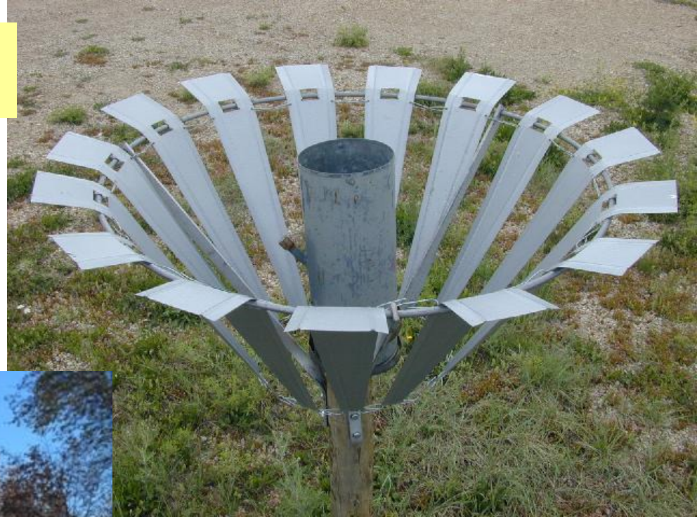
Right: Tretyakov Precipitation Gage at University of Colorado, Boulder
