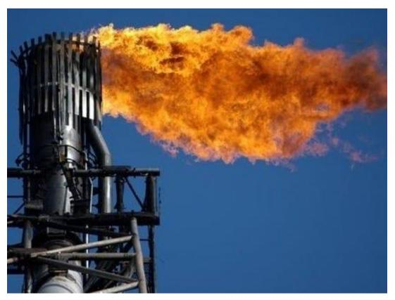
Excess methane is often burned off from oil and gas production and distribution systems. (Photo: Courtesy photo)
