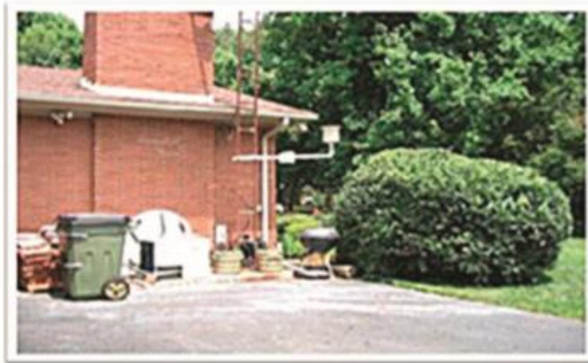
USHCN weather station at Hopkinsville, KY (Pielke et al., 2006). The station is sited too close to a building, too close to a large area of tarmac, and directly above a barbecue.
