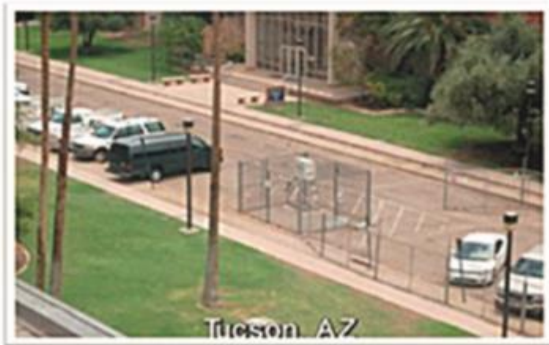
USHCN station at Tucson, AZ, in a parking lot on pavement. (Photo by Warren Meyer, courtesy of surfacestations.org .)
