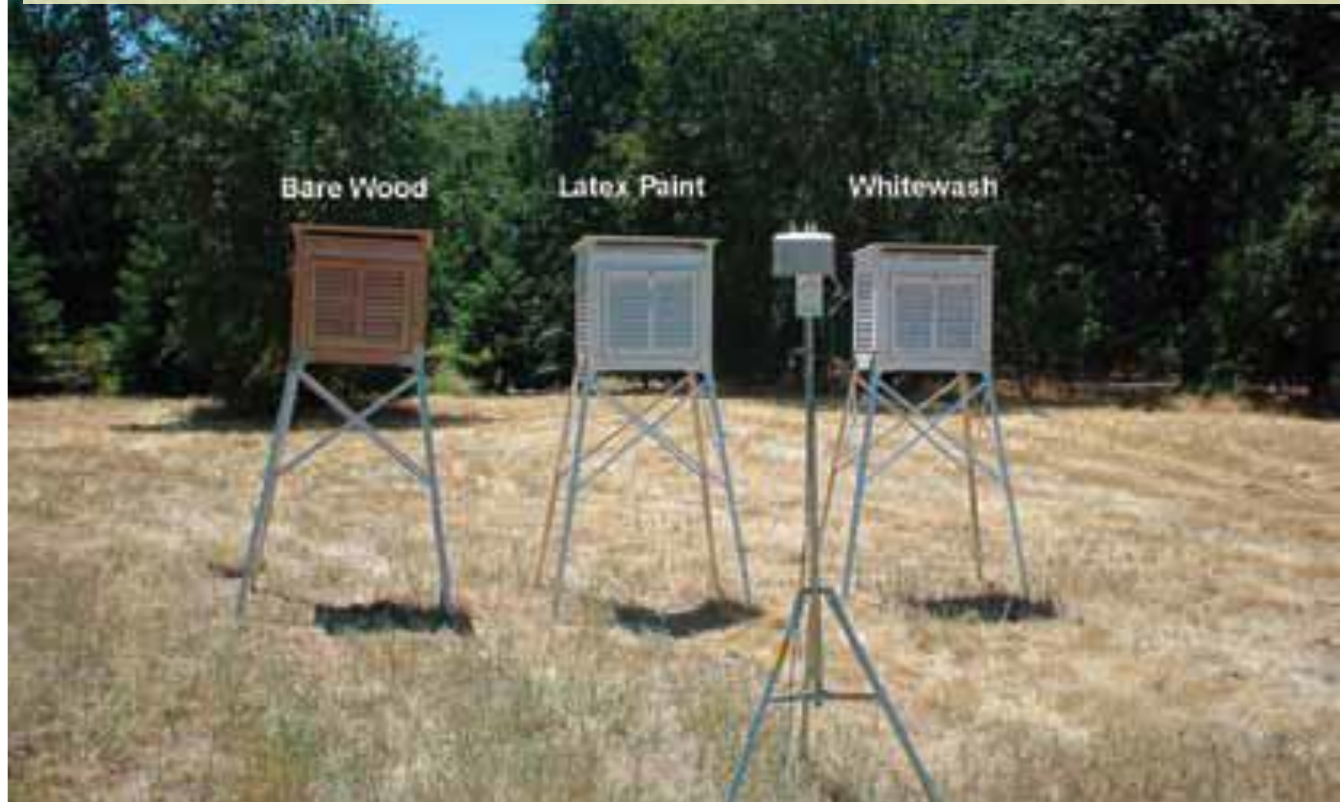
Three new Stephenson Screens as used by NOAA/NWS; stacked plate infrared thermometer
