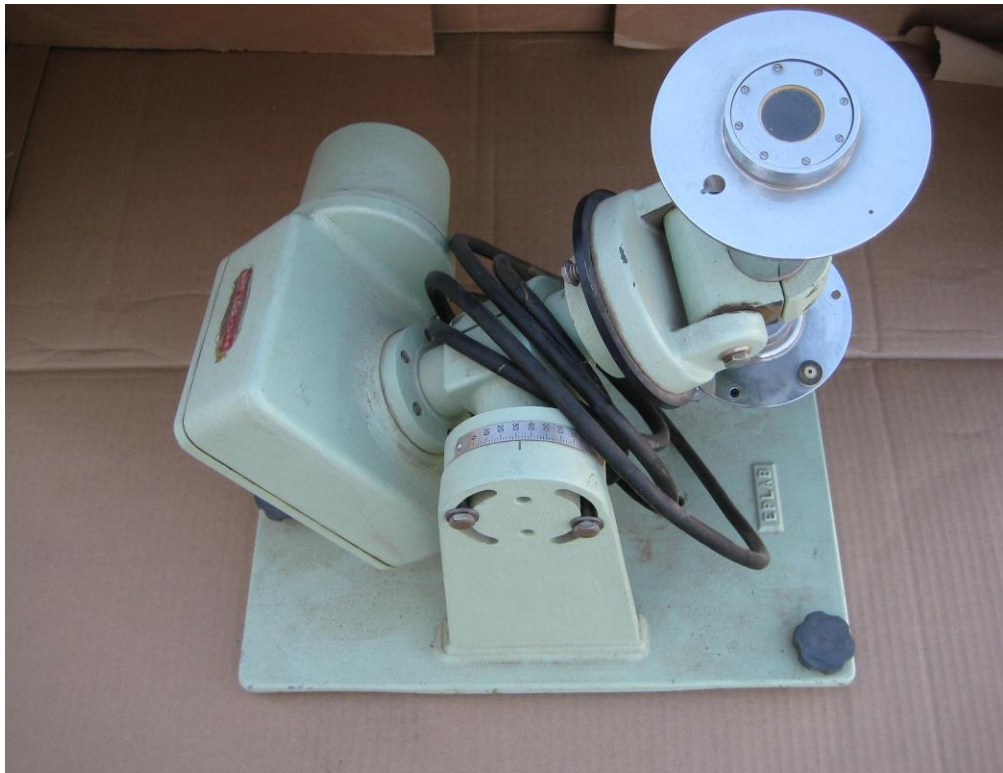
Figure 1. Picture of Solar Furnace Eppley pyrheliometer. Note the equatorial style tracking mount and clock drive.
