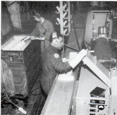
Airmen pulverize blocks of dry ice for fog seeding inside cargo hold of C-130. Drawing above shows pattern flown by planes upwind of airstrip so that the cleared area drifts over it.
