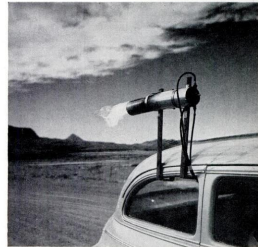
Generator on car creates clouds of silver-iodide smoke, seeding cloud formations in experiments to increase the rainfall
