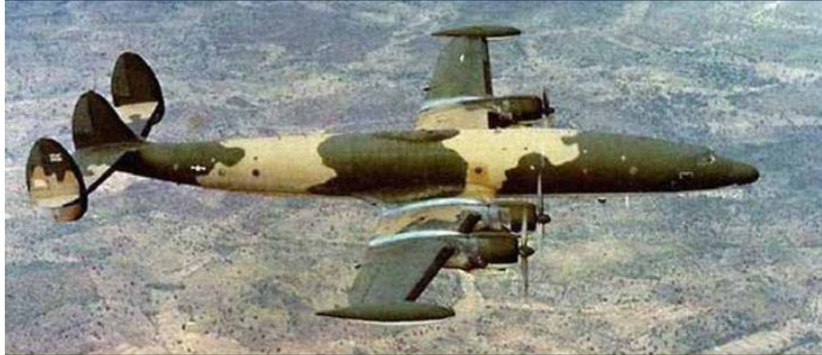
An EC-121R "Batcat" orbiting above the Ho Chi Minh Trail. The aircraft receives sensor signals and transmits the signals to Task Force Alpha's Information Surveillance Center, Nakhon Phanom, Thailand. (National Museum of the U.S. Air Force)
