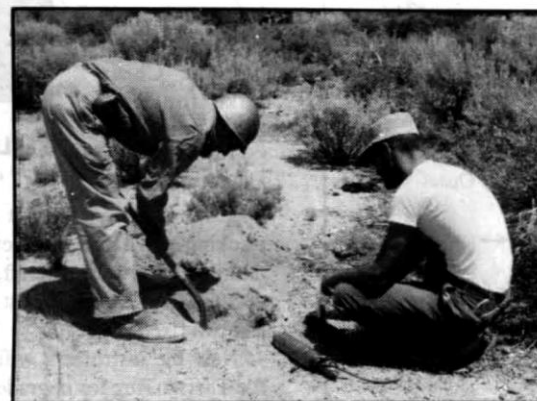
SEISMIC STUDIES —In July 1957, Dr. Pierre Saint-Amand and Gerry Malloy bury a geophone at Mono Lake to record shock waves.
