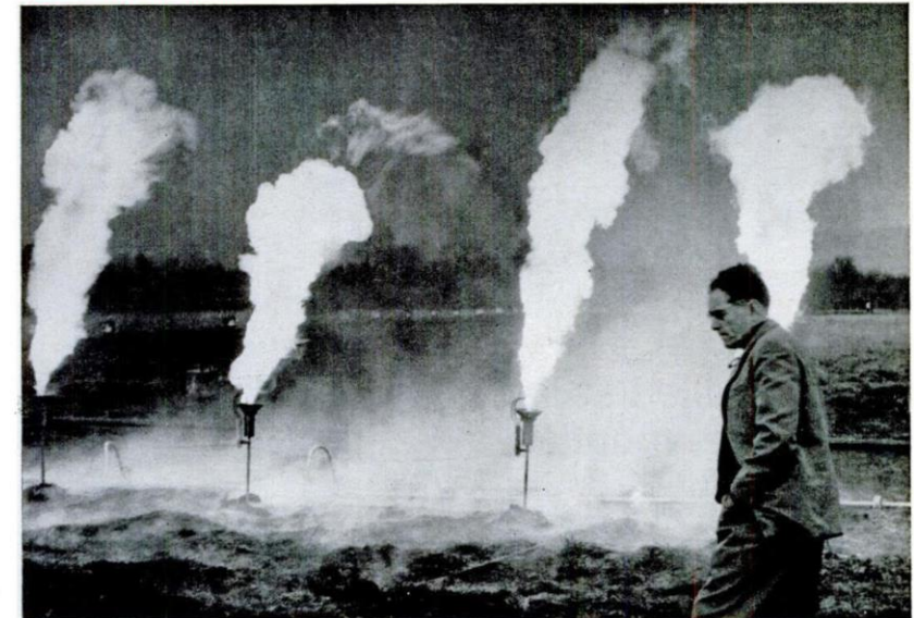
Lighted by glow of oil burners, Henri Dessens watches as heated air rises to form rain cloud.
