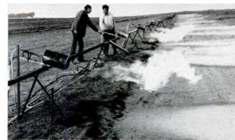
Liquid-propane burners heat air in fog-clearing tests. Natural gas can also be used. Future installations will be underground.
