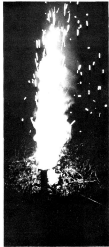
Ground-based silver iodide in acetone solution burner, top. Below, a pyrotechnic hygroscopic generator burns brightly from ground at night.
