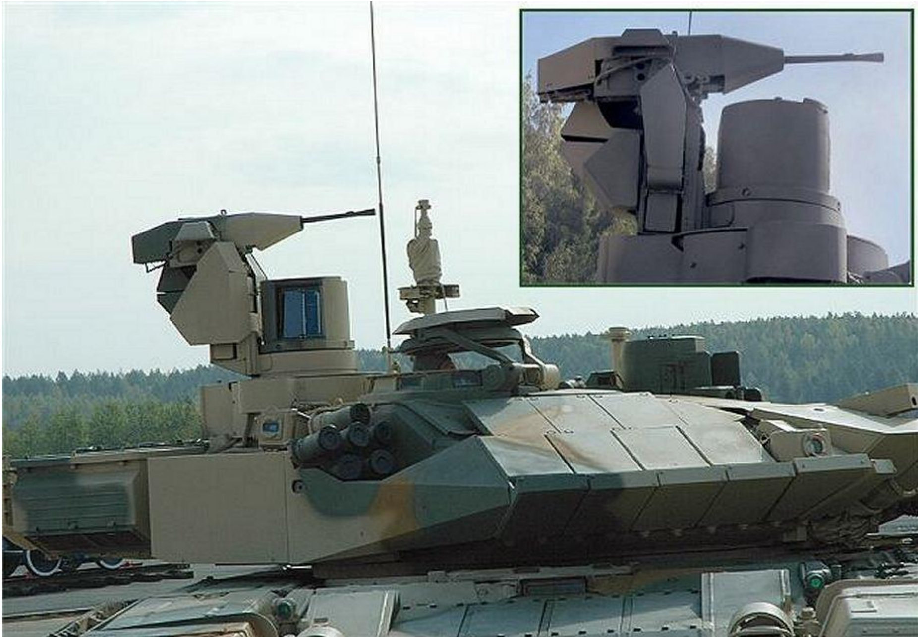
A remote-controlled weapon station armed with a 7.62mm machine gun is mounted on the top of the turret
