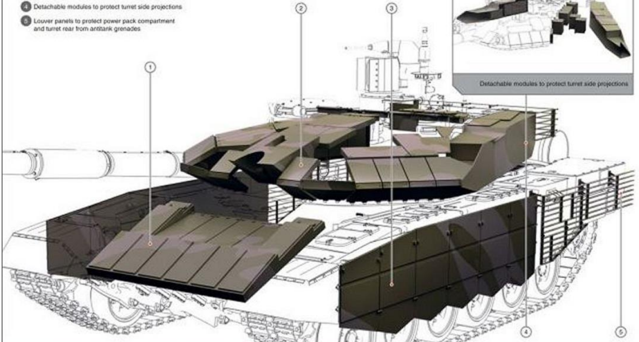
The hull and turret of the T-90MS are fitted with ERA (Explosive Reactive Armour) and wire cage armour.
