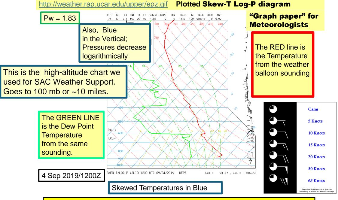
The Skew-T allows easy calculation of dozens of thermodynamic variables
