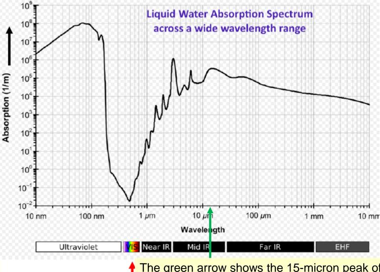
The green arrow shows the 15-micron peak of CO2 absorption and emission. Such radiation does not enter and warm the water.
