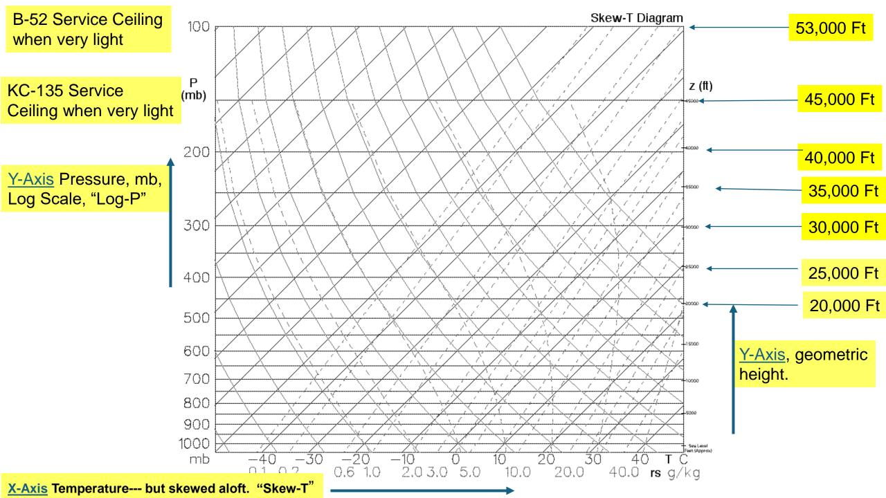
https://pielkeclimatesci.files.wordpress.com/2010/05/skew\_t.jpg SKEW-T LOG P DIAGRAM THERMODYNAMIC DIAGRAM AREA PROPORTIONAL TO ENERGY VERTICAL PROFILES OF THE TROPOSPHERE AND STRATOSPHERE 7.0-23 Height Scales This is the low altitude Skew-T [km and 1000's of ft] used by Army support units. Top only ~400 mb. ~23,000 Ft Mixing Ratio [g/kg] U.S. Standard Atmosphere [Temperature Profile] Moist Adiabats Dry Adiabats Isobars Isotherms Fahrenheit Temperature Scale
