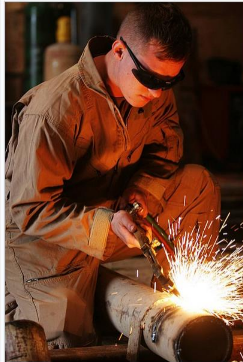
A cutting torch being used to cut a steel pipe
